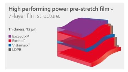
Exceed<sup>™</sup> XP, Exceed<sup>™</sup> and Vistamaxx<sup>™</sup> performance polymers boost the stretchability, holding force and toughness of the film:
