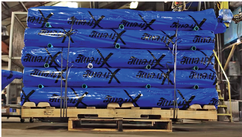
Tex-Trude is using Exceed XP 7 to produce 10-mil to 20-mil monolayer vapor-barrier construction films specifically designed for use under concrete slabs.
