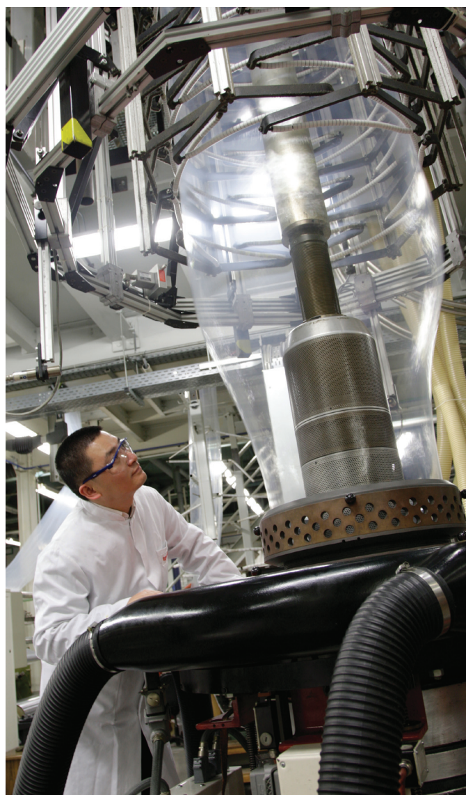
ExxonMobil's blown film testing at its Shanghai Technology Centre in China
