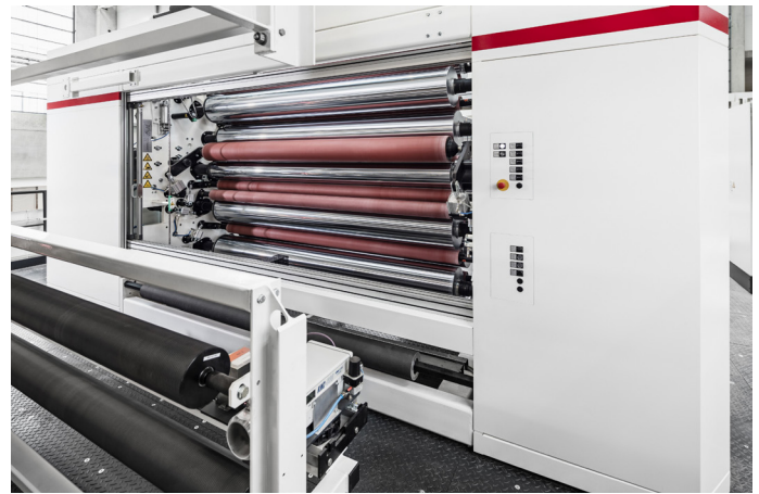
W&H 5L MDO line installed at Prepack's facility
