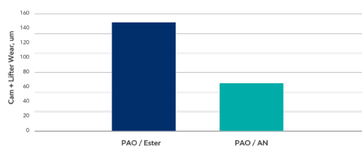
Sequence IIIIG Wear Performance of Experimental Low Phosphorus 0W-30 Engine Oils
