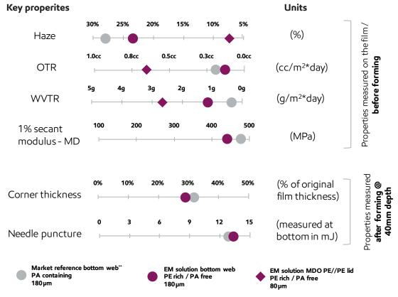
$<sup>\</sup>star\star$  PE/Tie/coPA/EVOH/coPA/Tie/PE with thickness distribution: 45/20/20/10/20/20/45, with 22% coPA and outer PE layer based on LLDPE and sealant PE layer based on Exceed m 1018. Data traceability: R2205-006953; R2209-009202
