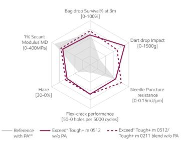
Oxygen transmission rate (OTR) less than 0.4 cc/(m2\*day) Water vapor transmission rate (WVTR) less than 6 g/(m2\*day). Data traceability R2301-011290. \*\*\*PE/Tie/coPA/EVOH/coPA/Tie/PE with thickness distribution: 24.2/6/6/2.6/6/24.2 with 16% PA
