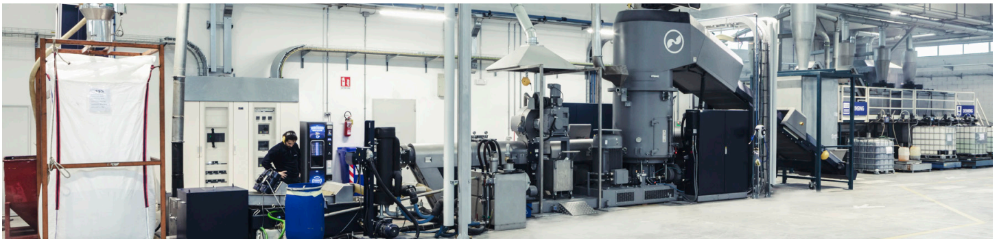
The recycling line at the Santa-Margherita plant, Italy where bags are sorted, washed, de-inked, and re-pelletized into a premium recycled product.
