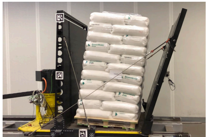
Pallets with Selene NextBag HDS which contain 50% PCR PE passed acceleration tests at ESTL, according to EUMOS40509.
