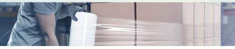
Exceed<sup>™</sup>, Enable<sup>™</sup> and Vistamaxx<sup>™</sup> performance polymers can create multilayer cast hand-wrap stretch films with excellent mechanical performance, while providing opportunities for significant raw materials savings.
