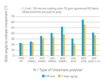
Slide angel test methods based on ASTM D-202
